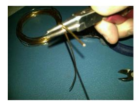
4) Continue to wrap the wire around the bottom tine until the end of the wire is facing away.
