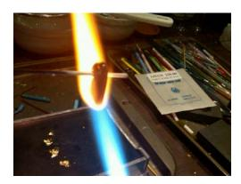
4) Rotate the mandrel until the glass wraps all the way around the mandrel and forms a nice round bead
