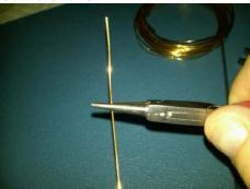
2) Next bend the top of the wire at a 90 degree angle.
