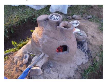
As you can see the front has an opening to reveal the hot coals, the top side openings are vents to help regulate heat, air flow and a work port. The center top opening is an annealing chamber. It worked quit well. Pictured below is the furnace in use.
