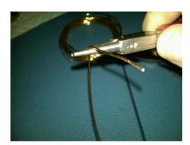
3) Then move the bent portion of the wire between the two tines of the pliers and bent the wire up and around the top tine of the pliers to start forming the loop.
